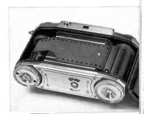
ture frame. Close the camera and set the frame counter (24) to the rhombus by means of the milled knob (25). Then turn the film winding knob (17) until it catches and the frame counter will show the number 1. The first frame is now prepared for exposure. Winding the film on by further turning the film winding knob (17) the frame counter will
