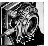
taneously with the release of the shutter, while the shutter itself opens 15 milliseconds (15/1000 sec.) later.
