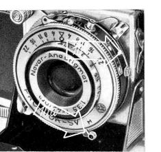
way by means of the shutter cocking lever (9). On the other hand the winding lever for the delayed action device (10a) has to be pressed over to the yellow dot on the shutter. As soon as the shutter release is operated, the clockwork of the delayed action device starts running. It releases the shutter automatically after about 8 seconds. The delayed action mechanism cannot be used when the shutter is set to "B".
