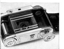
indicate the next figure and clearly show how many exposures have been made. The shutter is coupled to the winding mechanism so that the release knob cannot be actuated unless the film is wound on and the film winding knob (17) locks, thus obviating the risk of double exposure and blanks. It should, therefore, become a habit to adva**\text{Wewnerhancameras** are and after each exposure and to cock the shutter so that one is always ready for another exposure.
