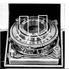
the depth of field only when the lighting conditions are favourable. To make short exposures in poor light the full aperture of the lens should be used, or as large a stop as possible. The CONTINA 24x36 mm makes work with large apertures easy, because the built-in range-finder prevents incorrect focusing and always provides for the exact distance between the camera and the subiect.
